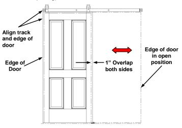
3.2. Lay out and mark the location of the holes on the wall. See Flat Track Head Section sheet. The end of the track and the edge of the door should be aligned. (see above)
